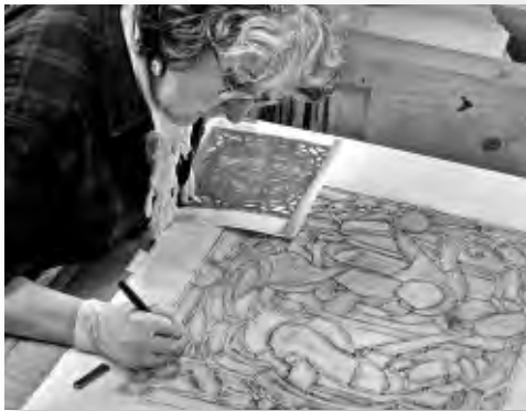
Master glazier Leslie Simonds refines a rubbing and compares it to a digital photo to ensure accuracy.
