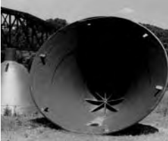
Hopper bells that form an airlock at the top of a blast furnace.
