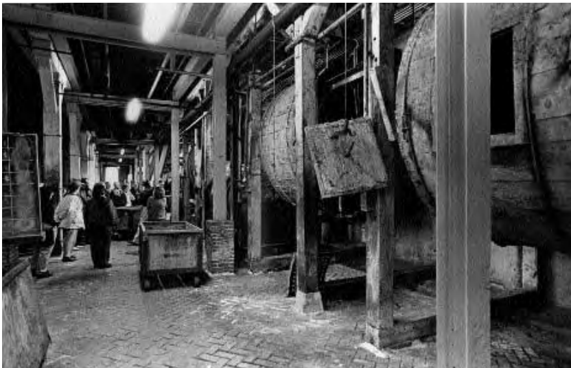
These large rotating drums, designed by Roy Kumer and made out of mahogany, were used to prepare the hides prior to grading and shipping.
